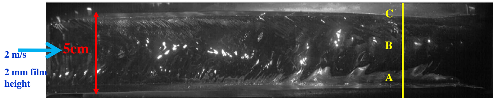
Inductive probe film height at 26cm downstream A: 6.0mm B: 7.8mm C: 10.0mm
