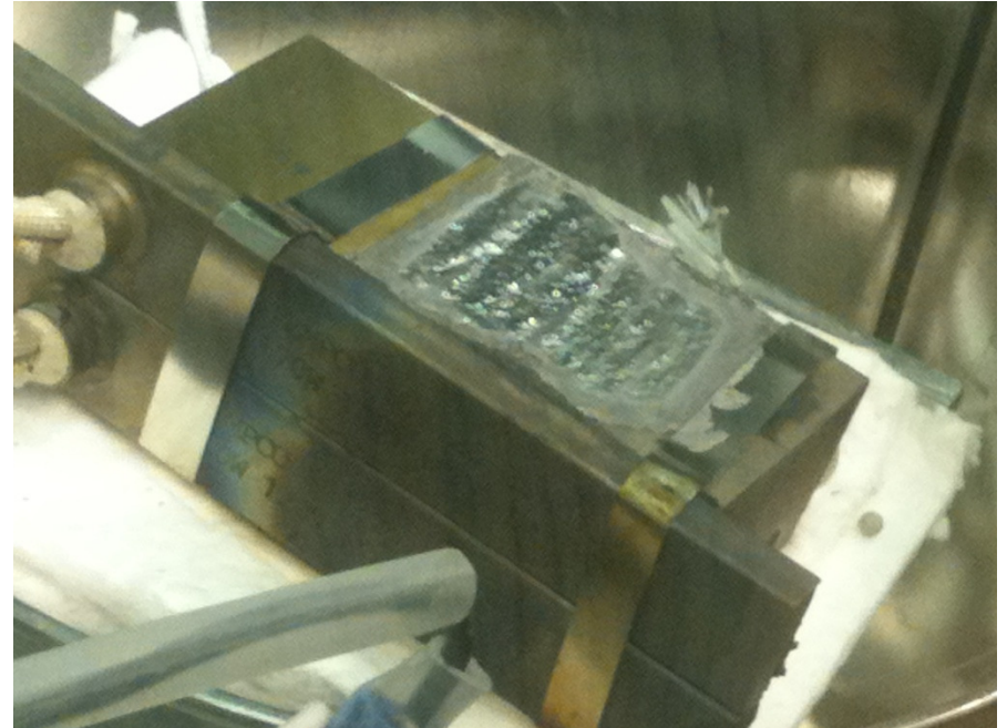
New LLD sample coated with a fresh layer of Li
