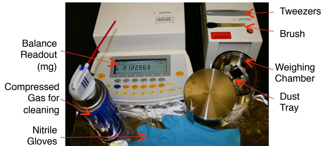
Microbalance 5 g capacity 1 μg readability
