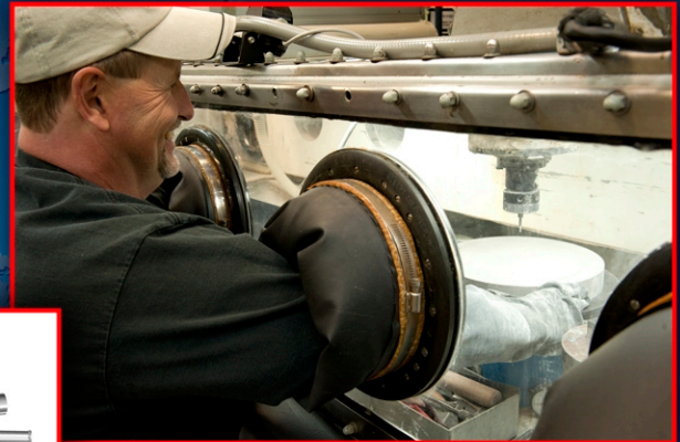
Inert Glove Box Machining of Li6 Material
