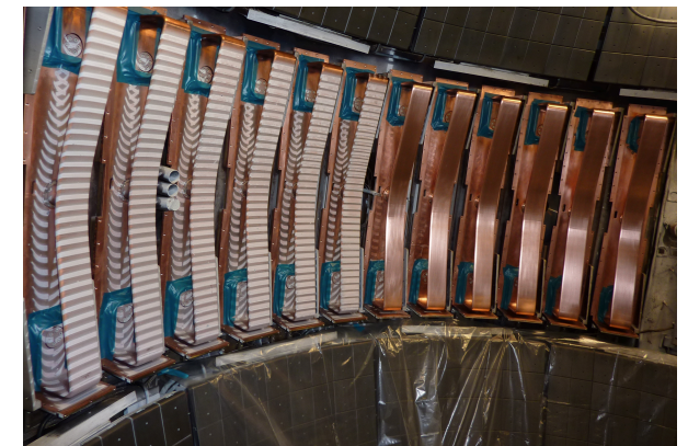
HHFW Antenna before and after cleaning
