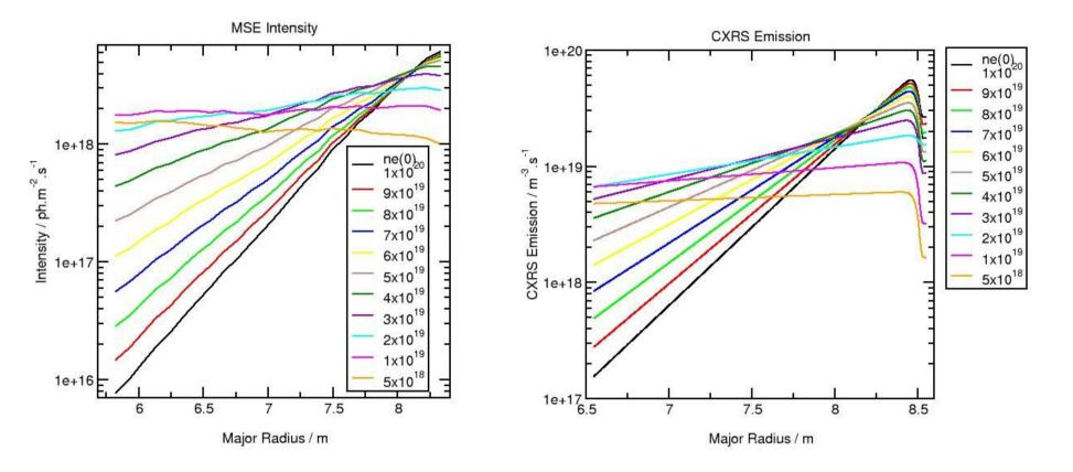
If the DNB can be operated in low density during the current ramp if will yield improved BES and CXRS signals—factor ~20 larger in both cases at the magnetic axis (R=6.5m).
