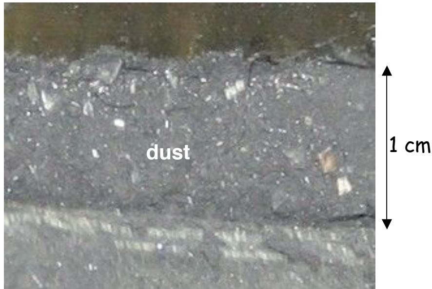
Dust in NSTX under lower divertor tile.
