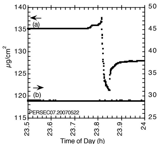
Fig. 1 Changes on (a) the upper and (b) the lower QMB. The excursion in (a) appears to be due to mechanical relaxation.
