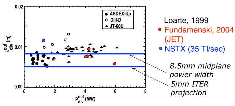
Fig. 5. Measured power deposition width versus divertor power for H-mode discharges without gas puff in the ITER power deposition database. (Mapped from strike point to outer mid-plane.)
