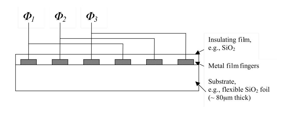
Three-phase electrostatic bucket brigade to move dust particles.
