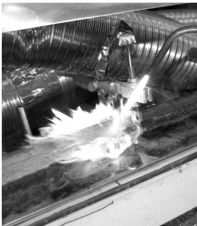
Fig. 1 Reducing Flame Dissociating Tin, Silver and Copper Oxides
