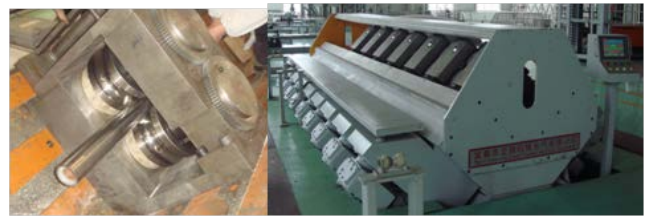
Figure 7 Pair of Compaction Rollers and Compaction Machine
