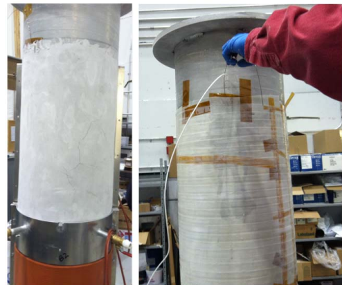
Fig. 7. Full Diameter Test Left: After Baking, Right: During Washing Note use of preplaced wire to facilitate removal
