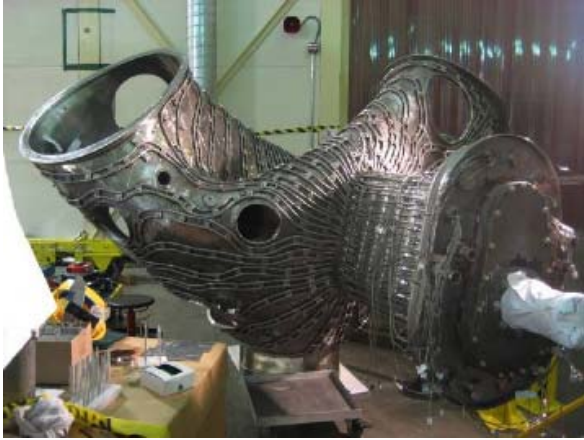
Fig. 5. Vacuum vessel sector with installed services.
