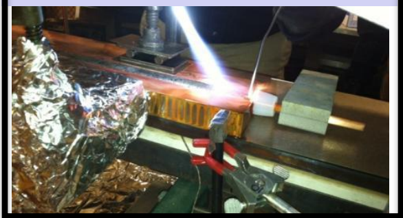
Cooling tube soldered with resin-based flux into inner TF conductor
