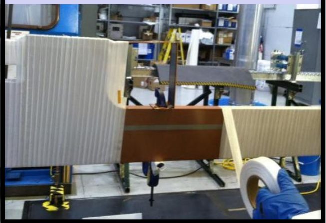
Conductor being wrapped with fiberglass insulation
