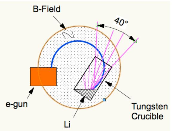
Crucible orientation to coat upper divertor. Ratio of crucible depth to opening is 2:1 and allows a 40 degree spray.
