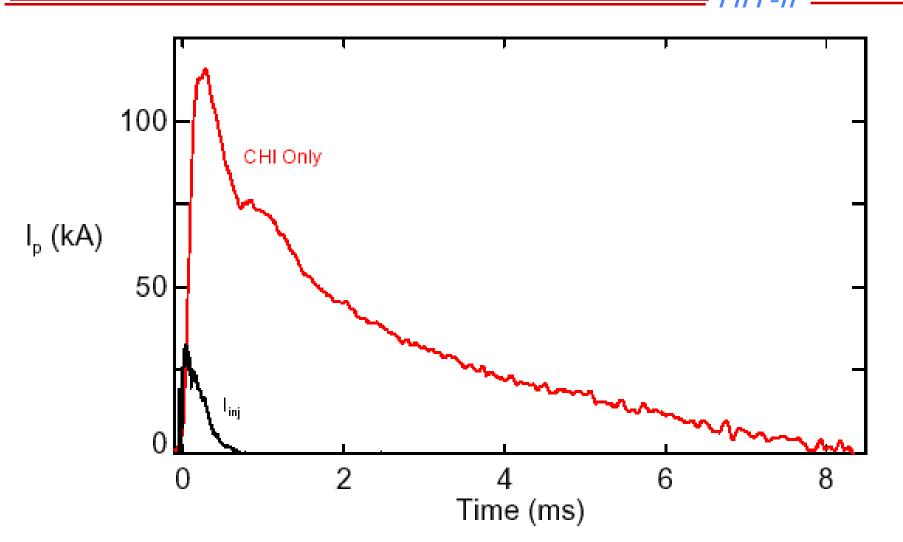
Note the persistence of CHI plasma current after the injector current has been reduced to zero
