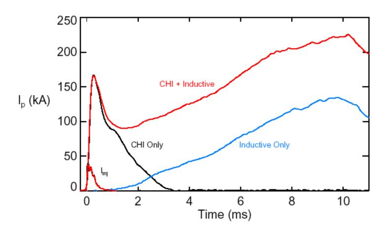
Both discharges have identical loop voltage programming
