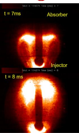
Expect axisymmetric reconnection at the injector to result in formation of closed flux surfaces
