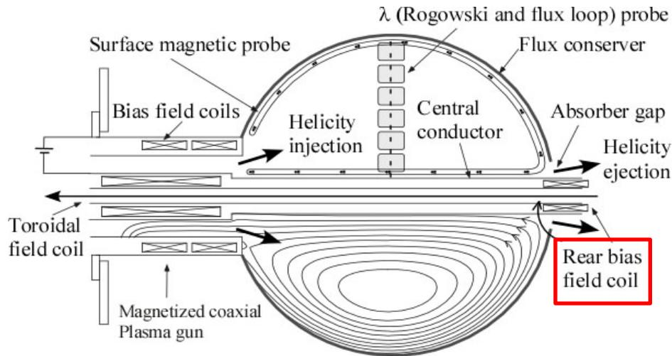
■ As the ejected plasma contacts the rear gap of the FC or after the kink instability occurs, the injection current flows between the FC and the central conductor due to the arc discharge on the gap (Absorber arc).
