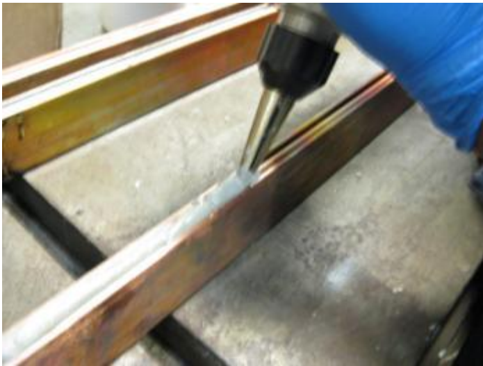
Solder paste injection over cooling tube
