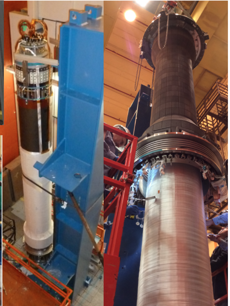
CS casing installed over the TF/OH coil bundle
