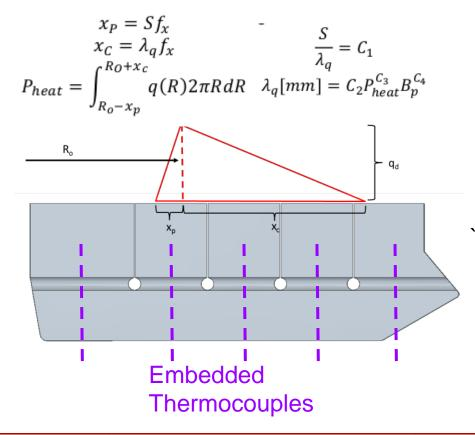
$$\begin{aligned} x_p &= C_1 C_2 P_h^{C_3} B_p^{C_4} f_x \\ x_c &= C_2 P_h^{C_3} B_p^{C_4} f_x \\ \underline{\text{Take 3 shots, A, B, C}} \\ C_1 &= \left( x_p / x_c \right)_i \\ \ln(x_c / f_x) &= \ln C_2 + C_3 \ln P_h + C_4 \ln B_p \end{aligned}$$
