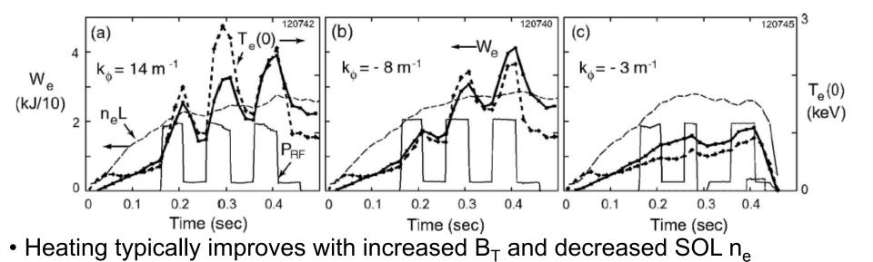
Suggests that poor heating efficiency results when fast-wave cutoff is too close to antenna
