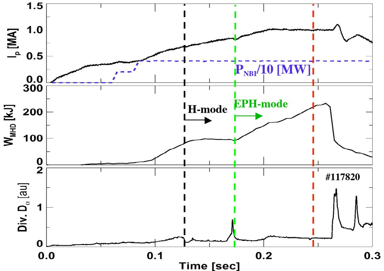
Fig. 1 – temporal evolution of the Enhanced Pedestal H-mode. The colored dashed lines represent the kinetic profile times in Fig. 2.
