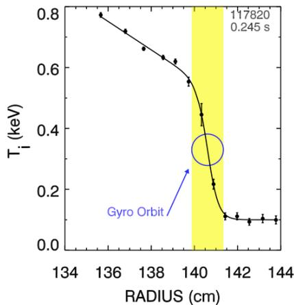
Fig. 3 – comparison of the  $T_i$  profile and poloidal ion gyro-diameter.
