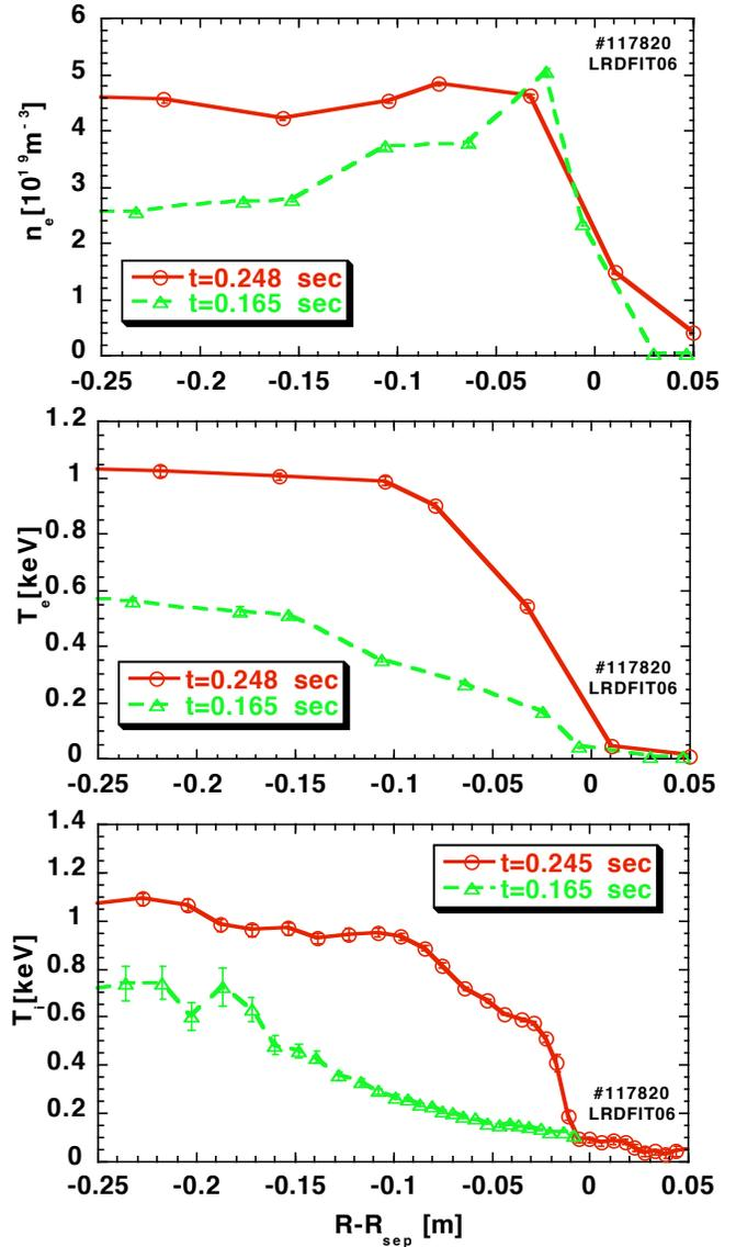
Fig. 2 – Profile comparison during the regular H-mode phase and the Enhanced Pedestal H-mode phase from Fig. 1.
