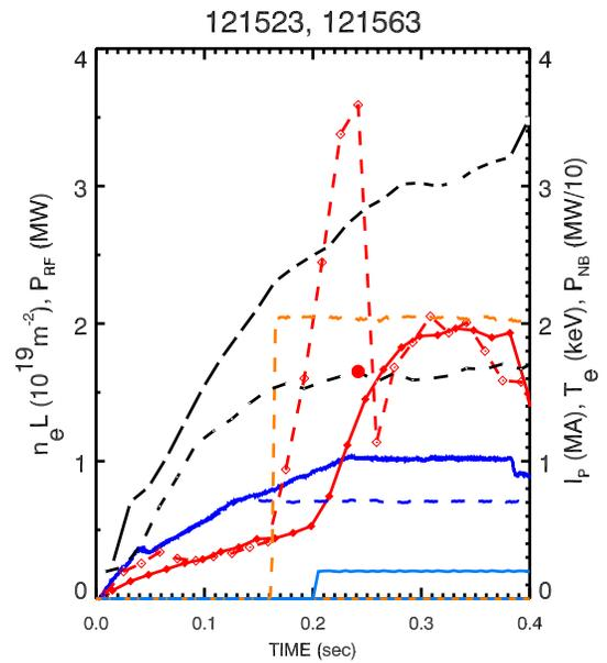
Comparison of profiles and peak trajectories for a good RS shot from XP 610 (RS) and a good shot from XP 617 (HFW). While the RS shot achieved higher pressures due to density, the HFW discharge reached higher  $T_e$  with sharper core  $T_e$  gradients with stationary  $n_e$  profiles. To diagnose fluctuations with correlation and profile reflectometers, the  $n_e$  profile must be monotonic (L-mode), with the peak lower than  $2 \times 10^{19} m^{-3}$ .
