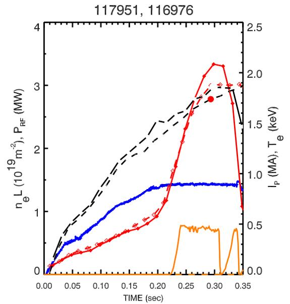
Comparison between shots from B. LeBlanc's XP 538 (RS with HHFW at 4.5kG) and its reference shot from XP 522 (RS). About 700kW of HHFW was injected (best shot). Locked modes were an issue and RF coupling was an issue. Nonetheless, somewhat higher temperatures than the reference shot were reached.
