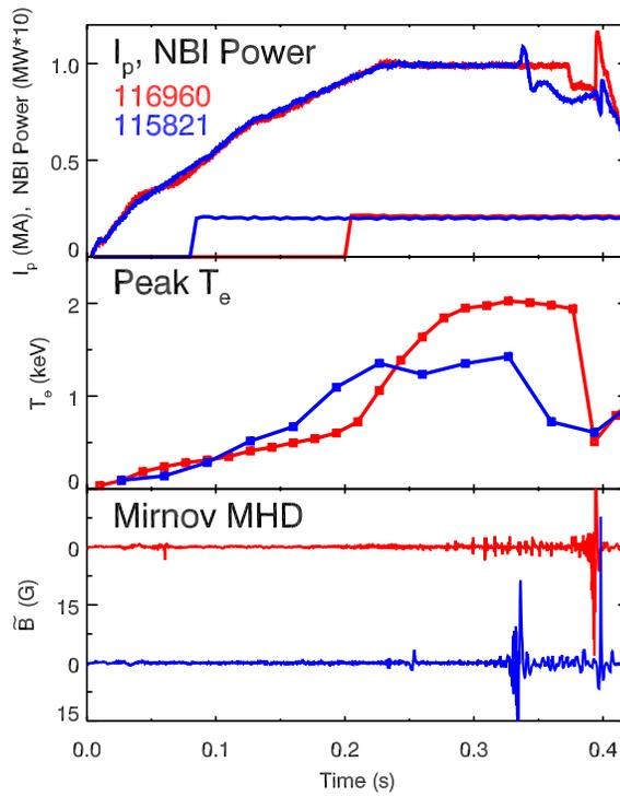
Results from XP 522 & 610 comparing reversed shear vs. flat core  $q$ -profiles. Note that beam timing was the primary input difference between the two discharges.
