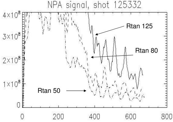
TRANSP shows modulations at all tangency radii that match the beam modulations. This is not seen in the measured NPA signal, particularly for Rtan 80, near the magnetic axis. (The measured NPA signal is not shown)
