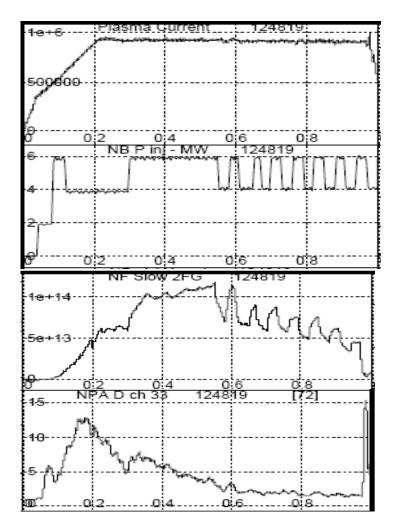
Shot 124819 is from XP 737. However, the NPA channels show no correlation with the beam modulations and neutron signals, even at the highest channel. This may be due to the NPA sightline viewing outside of the beam deposition region. The expectation is that if the NPA sightline is adjusted, the modulations will be visible.
