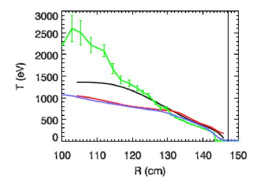
It is not yet clear that the ion temperature measurements are correct. If they are, they require anomalous ion heating, to prevent  $\chi_i < 0$ .
