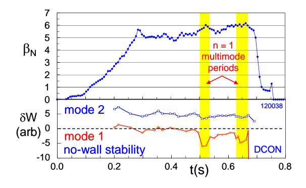
Figure 1: Ideal MHD stability for the two least stable n = 1 modes (NSTX discharge 120038). The vertical bands indicate where the  $2^{nd}$  least stable mode is expected to have a greater response to external stimulus than the least stable mode.
