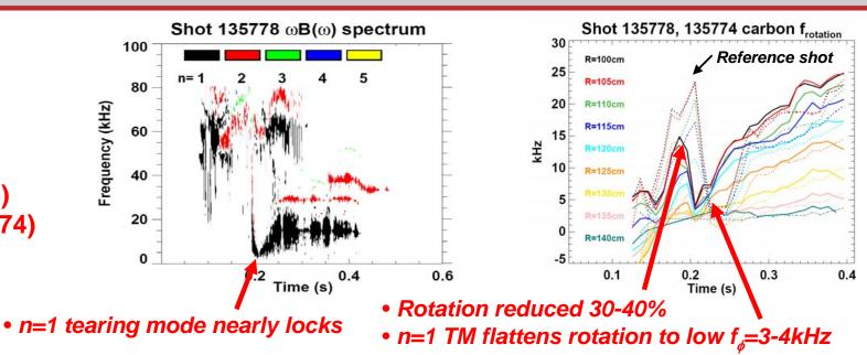
• Optimal corrective n=1 field (135779) vs. reference (135774)
