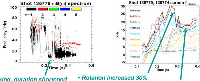
• n=1 tearing delayed, no locking, duration shortened
