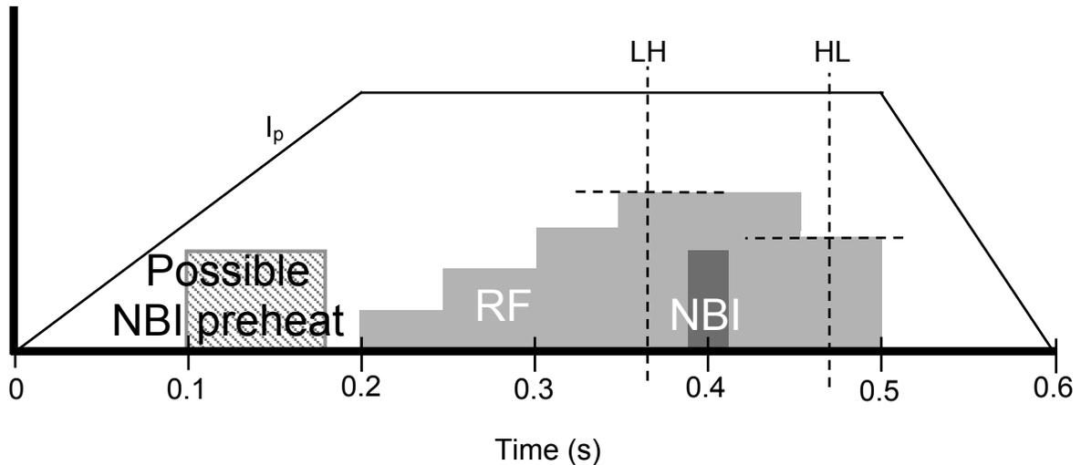
**Figure 3** Timing and shape of  $I_p$ ,  $P_{RF}$  and  $P_{NBI}$  for the second target discharge
