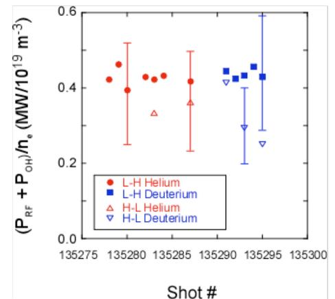
**Figure 1** Ohmic heating plus the electron heating from RF normalized to the line-averaged density for D and He plasmas (XP941).
