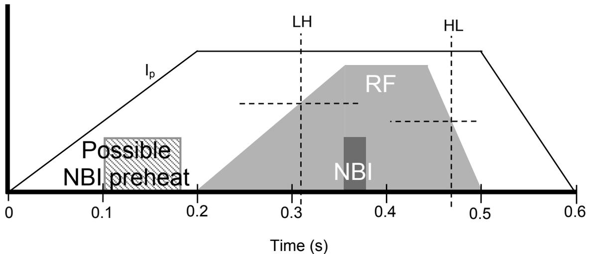
**Figure 2** Timing and shape of  $I_p$ ,  $P_{RF}$  and  $P_{NBI}$  for the first target discharge
