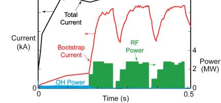
> Up to 2.7 MW of  $k_{\phi} = -8 \text{ m}^{-1}$  heating, produced transient H-mode
