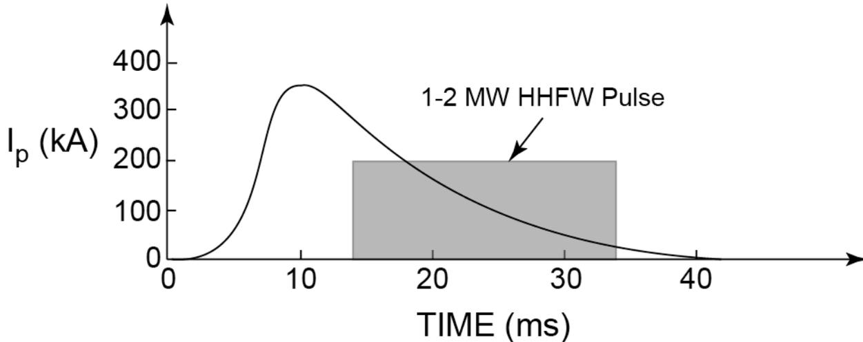
**Figure 1:** Schematic showing time of the 20 ms HHFW heating pulse relative to the time evolution of  $I_p$ .
