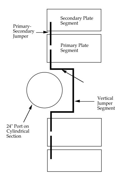
The jumpers between primary and secondary plates are short and simple.
