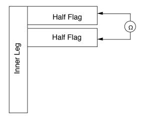
Resistance measurements were made on all 36 upper and 36 lower, total 72 joints, after initial center stack assembly on 10/6/98 and again during the past outage on 5/25/00 when the center stack was removed from NSTX. Data is given on the attached spreadsheet (courtesy of J. Chrzanowski and J. Gething, who took the measurements).
