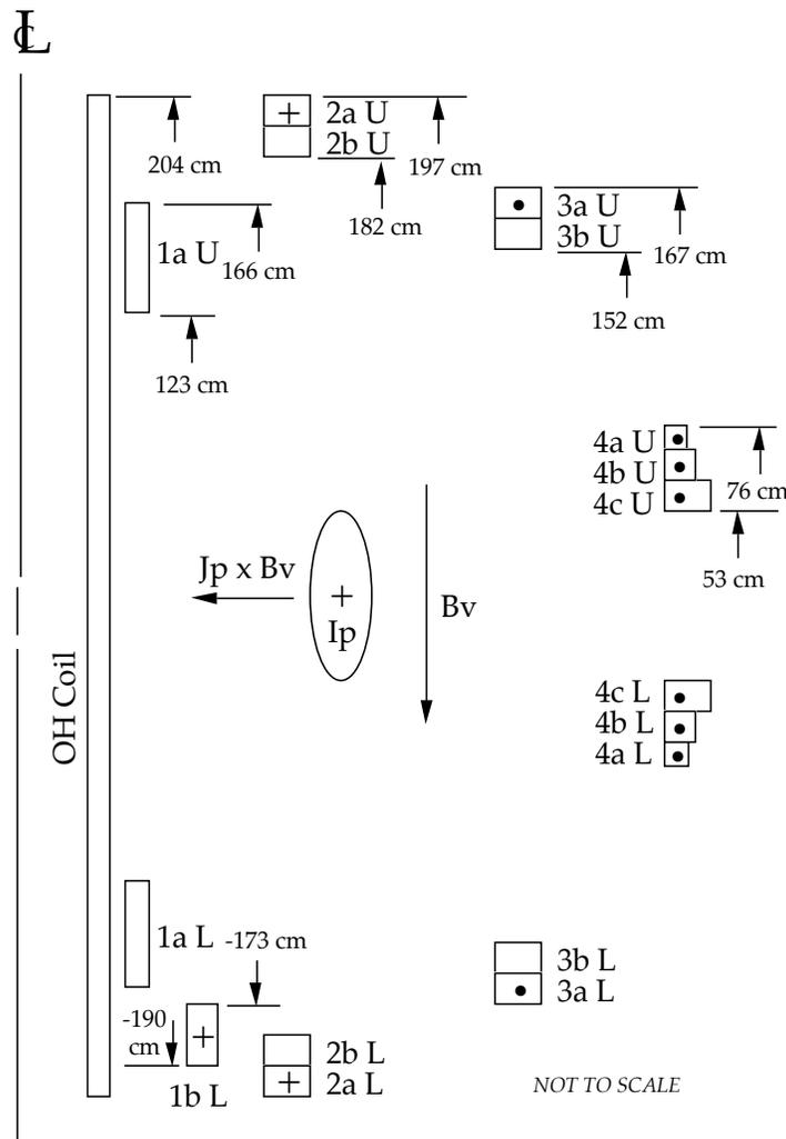
Based on guidance from physics the plasma was modeled using two current filaments at  $r=91.5$  cm and  $z=\pm 21.7$  cm, with the current set to 1.0MA in which ever filament produces the worst case force, and to zero in the other.
