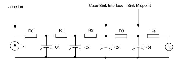
To determine R0, R1, R2, and C1 values, a curve fit procedure was used against the published transient thermal impedance curve for the device. Semi-log and linear curves showing a comparison between the response of the model and the published data is given in the following two figures.
