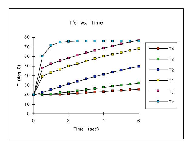
Since both the thyristor junction temperature and resistor temperature remains well below 100C, it is concluded that the 5.0 second pulse is feasible.
