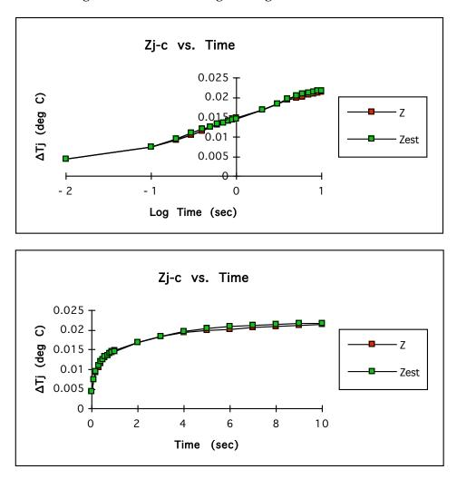
The SCRs are clamped to a water cooled heat sink on one side and a solid copper block on the other. To facilitate a simple simulation of the effect of these heat
