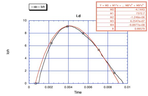
A curve fit to the OH current waveform over the interval of interest was made as follows...
