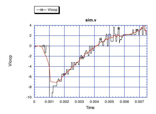
The discretization and noise associated with the current measurements cause the significant fluctuation in the simulated voltage signal.
