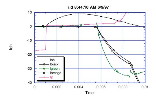
The negative plasma current measurement prior to 1mS is assumed to be an instrumentation anomaly (probably integrator drift which is resent at t = 1mS), so it is ignored. It is noted that the plasma current begins at t = 7.25 mS (small
