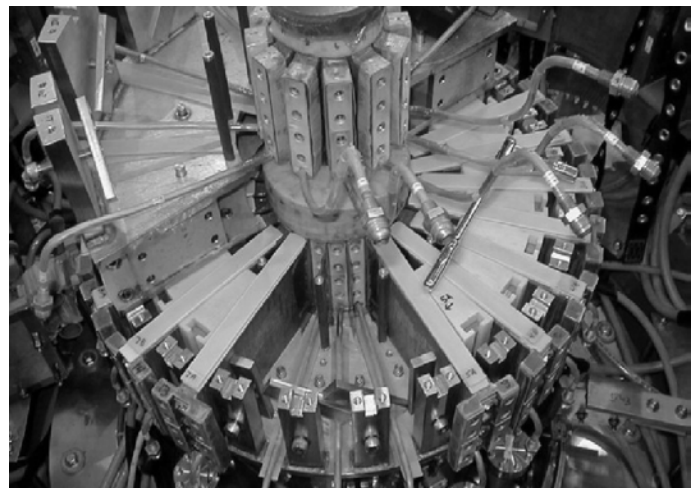
Fig. 3. G-10 Wedges and Shims of Original Assembly
