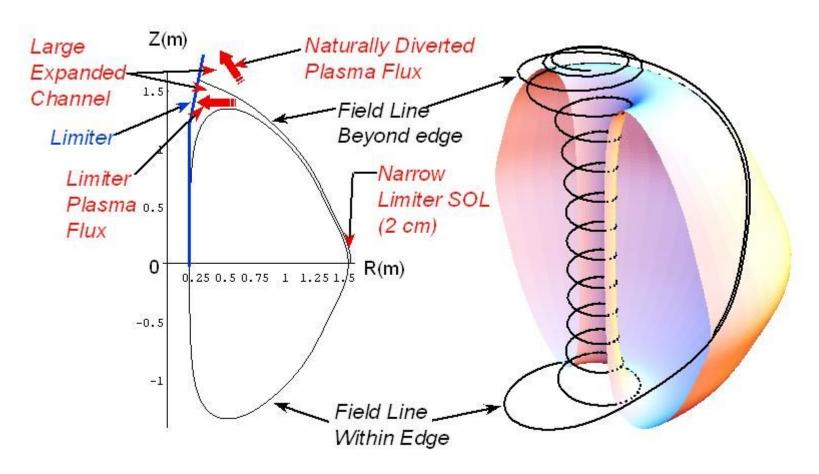
**DIII-D observed H-mode confinement in inboard-limited plasmas**
