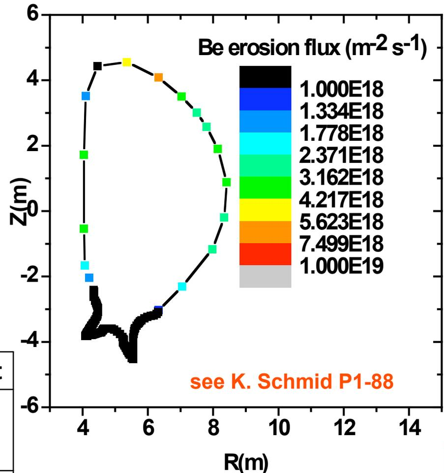
Erosion of Be first wall may become a lifetime problem for inhomogeneous loading
