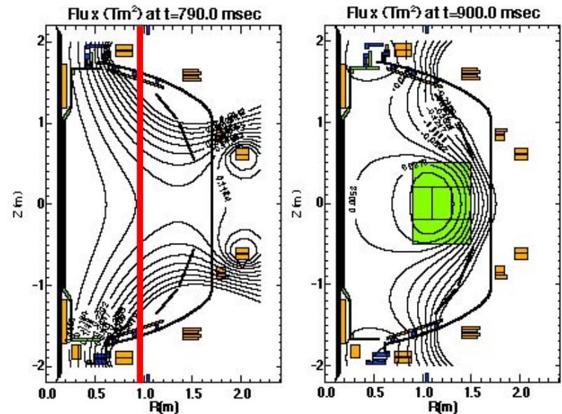
Ramp-up at large  $R \rightarrow$  limited to  $I_p = 160$  kA
