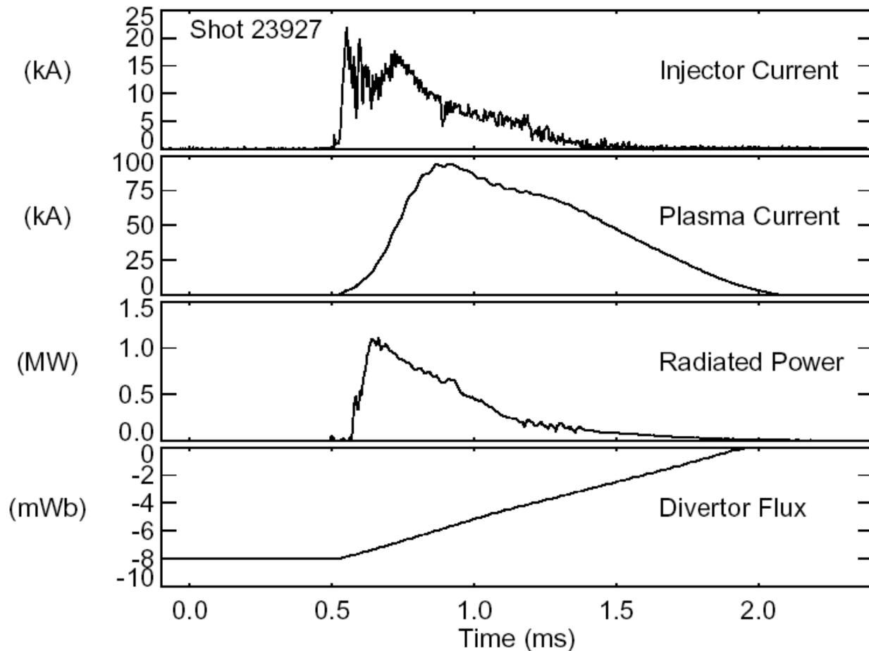
CHI only discharge: After the injector current is reduced to zero, substantial plasma current still remains. This can only result from the presence of a closed field line plasma configuration. This closed field line plasma configuration is used as the target for the inductive ramp.
