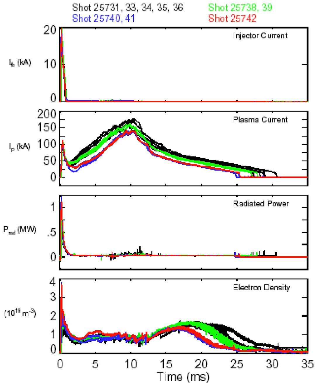
Under gas loaded wall conditions, good coupling to induction can be regained if gas injection for CHI formation is reduced
