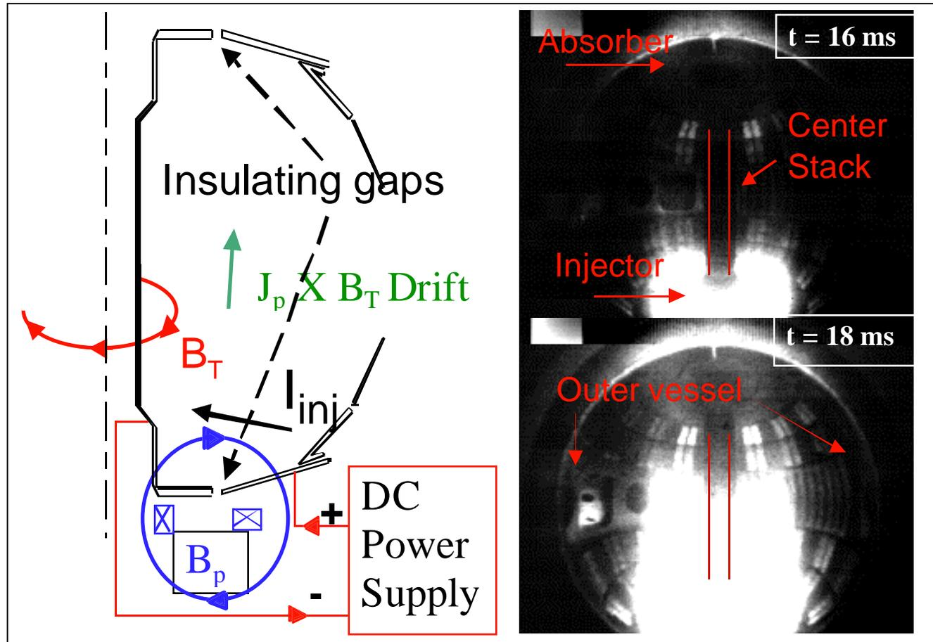
Expect reconnection processes to redistribute edge current to the interior, forming closed surfaces
