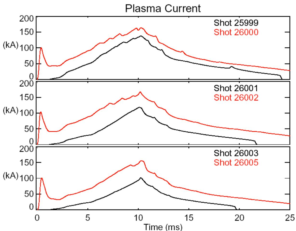
Coupling to induction reduces at higher CHI plasma densities, which results due to reduced wall pumping during later shots
