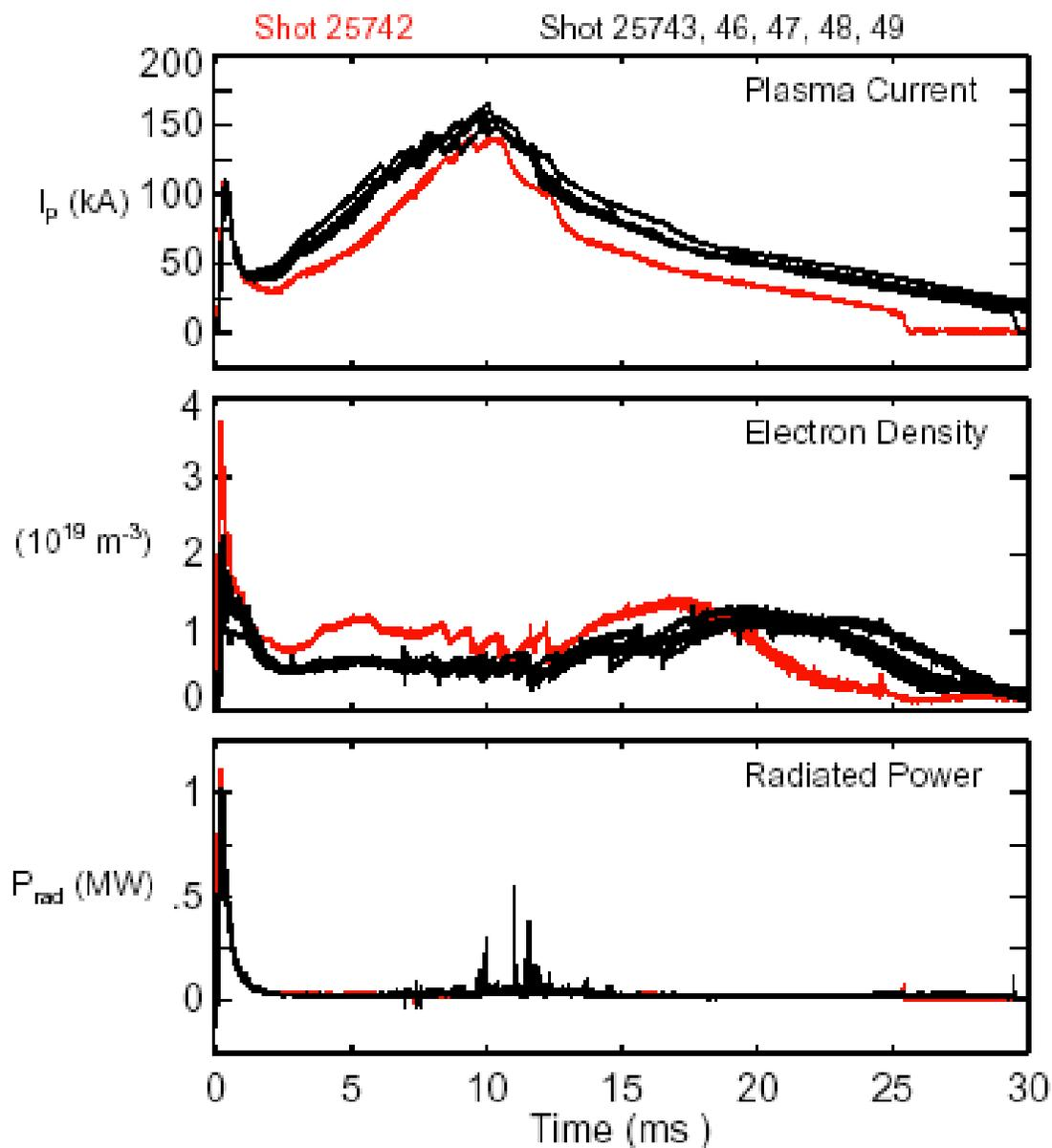
Highest ever plasma current (265kA) obtained using CHI start-up. Discharges can be now *initiated* and maintained *in a diverted configuration*
