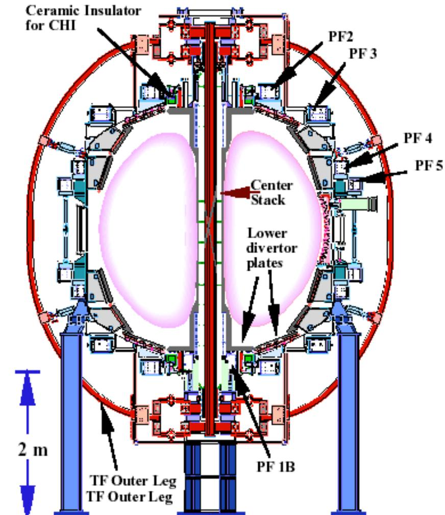
CHI injects toroidal flux linking poloidal flux ( $\dot{K}_{inj} = 2V_{inj}\psi_{inj}$ )
