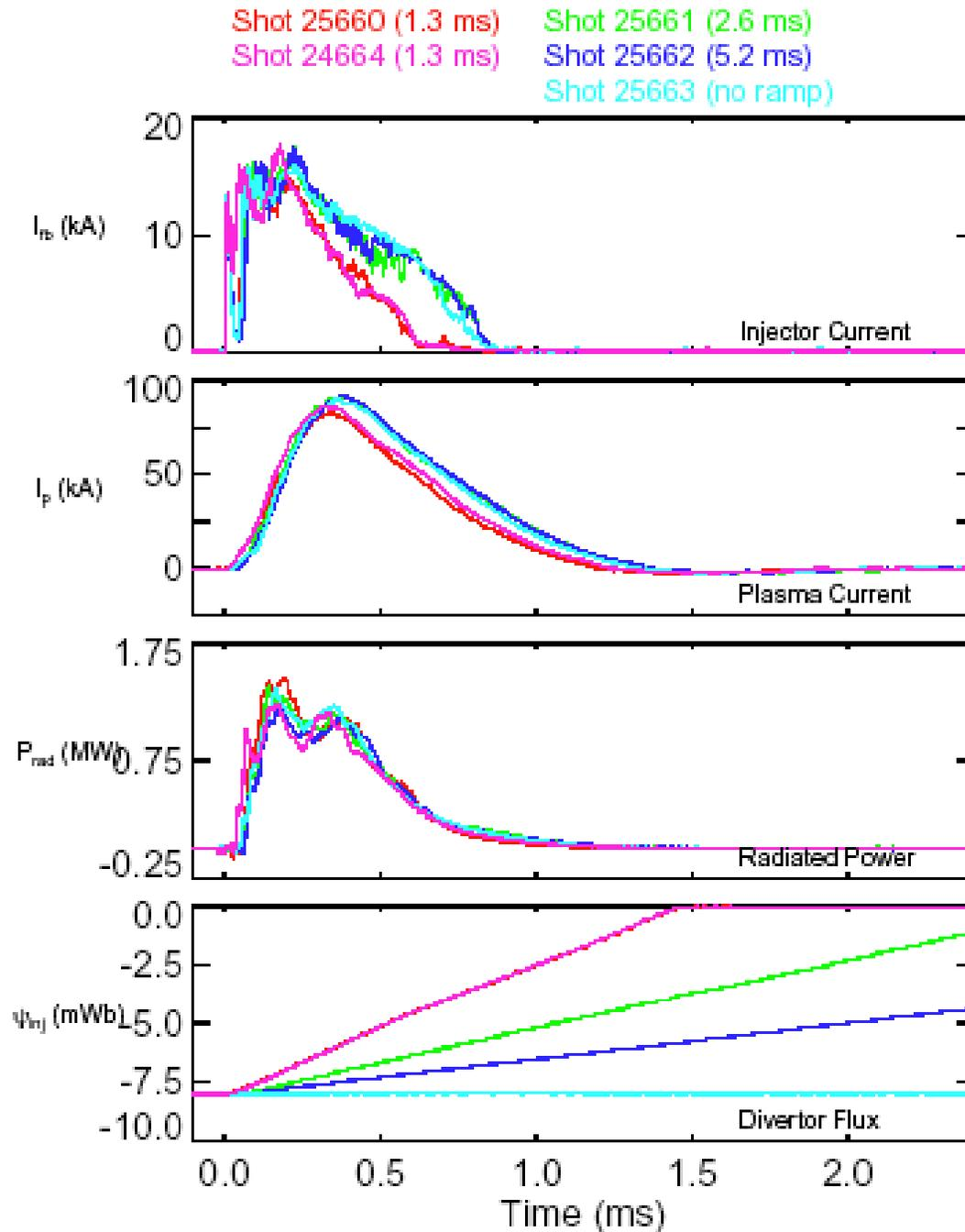
CHI started discharges without divertor coil ramp-down also outperform inductive only discharges and are similar to discharges produced using divertor coil ramp-down
