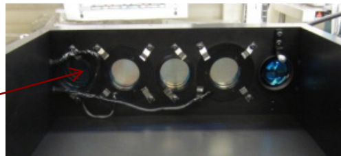
Single sightline, 4 wavelength polychromator prior to installation in MSE rack
