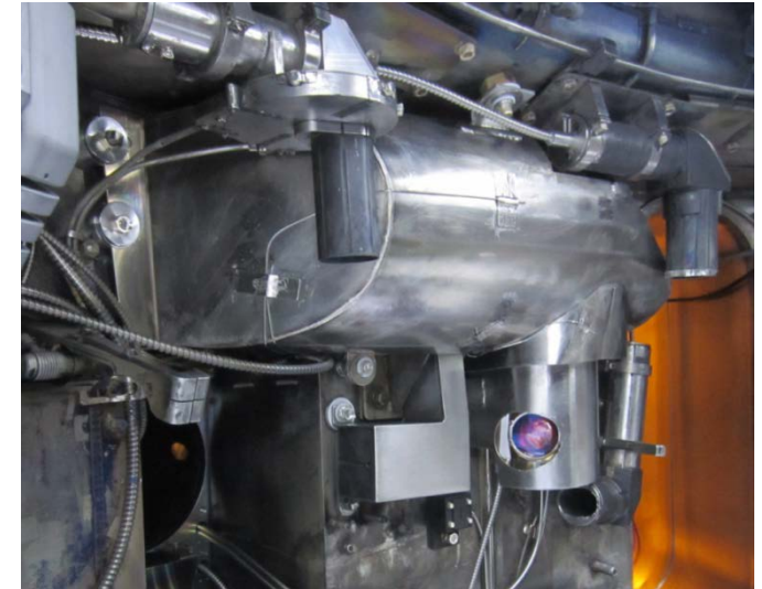
MSE periscope covered with radiative heat shield
