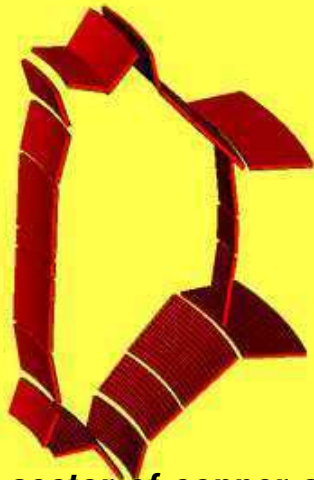
One toroidal sector of copper stabilizers (8728 triangles)
