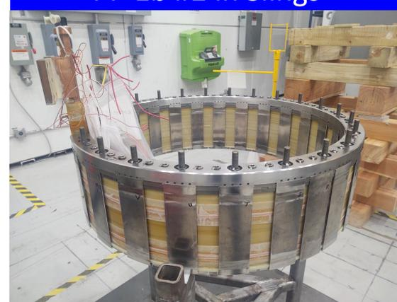
One bay w/ a complete set of new welds, brackets, "biscuits" & toroidal blocks
