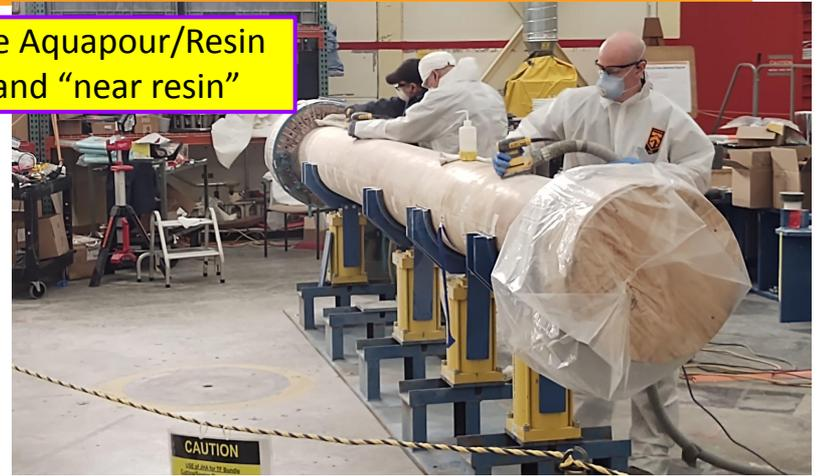
Fully Sanded and Cleaned Toroidal Field Bundle
