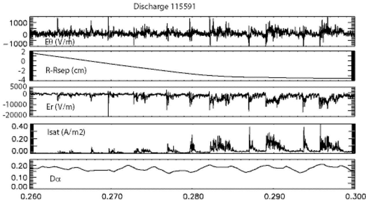
Probes measure ELM plasma parameters with high (1 MS/s) time resolution.
