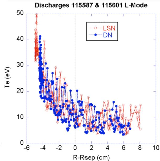
L-Mode LSN and DN, 800 kA, 1.2 MW NBI, 2 MW Pin,  $n_e \sim 2.2 \cdot 10^{13} \text{ cm}^{-3}$
