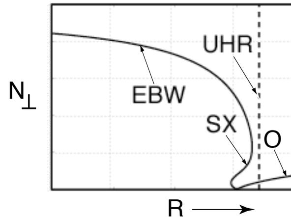
$$T(N_{\perp}, N_{\parallel}) = \exp\left\{-\pi k_o L_n \sqrt{(Y/2)} \left[2(1+Y)(N_{\parallel, \text{opt}} - N_{\parallel})^2 + N_{\perp}^2\right]\right\}$$
