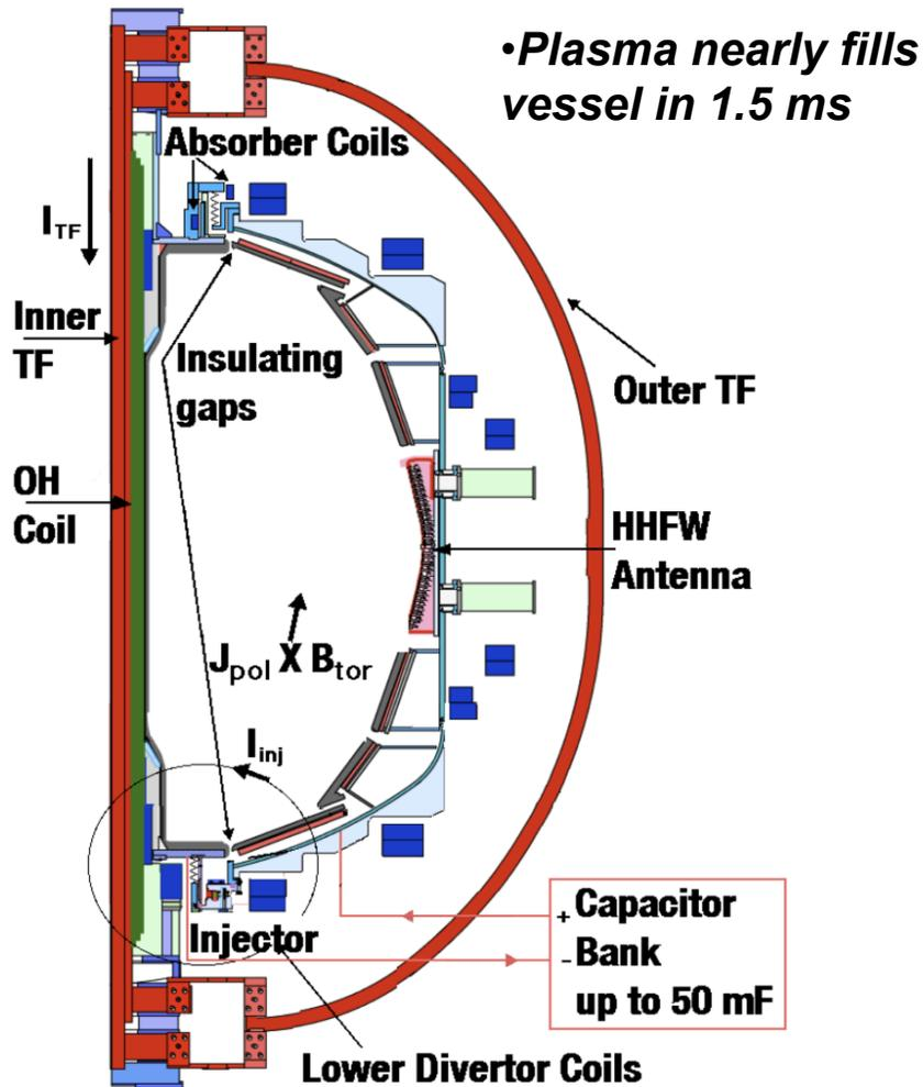
•The limited space for the center column in an ST necessitates alternative start-up and current drive.
