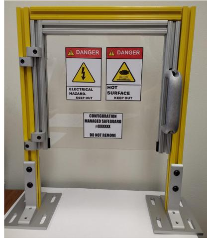
**3: Safety Instrumented System** - Dual PLC system used to turn off NB, FCPC power to test cell in the event of door violation, emergency stop, etc.
