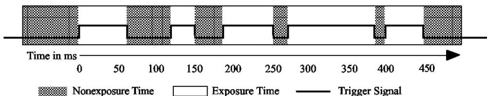
In `BULB_MODE`, `pl_exp_start_seq` calls the setup. The camera enters clear mode while it waits for a **true** external trigger signal to start each exposure. The CCD continues to expose until a **false** trigger signal ends the exposure. In the diagram above, the trigger signal line moves up to represent a **true** trigger and down to represent a **false** trigger.
