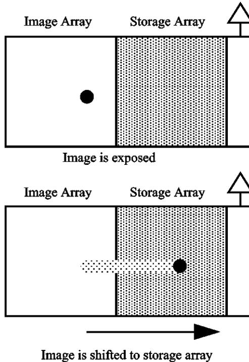
Although the frame transfer time is usually only a few milliseconds, smearing cannot be eliminated when the shutter is left open for the entire sequence. The higher the ratio of the *exposure\_time* to the frame transfer time, the brighter the image is in comparison to the pattern caused by smearing. An *exposure\_time* that is too long will saturate the pixels and cause the image to lose all contrast.
