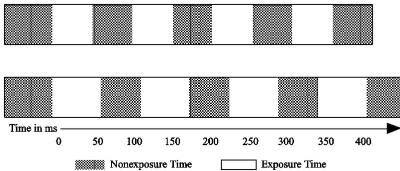
The first sequence runs with a filter that uses exposure and nonexposure times that are equal. In the second sequence, the exposure time is longer, but the time between exposures remains the same as in the first sequence.
