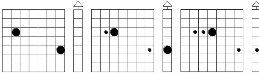
In most frame transfer applications, the shutter opens before the sequence begins and closes after the sequence ends. The charge gathered during the shift creates a smear across the image array.
