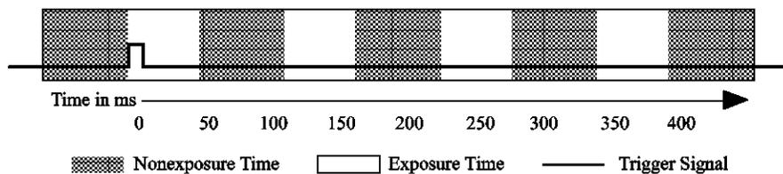
In `TRIGGER_FIRST_MODE`, `pl_exp_start_seq` starts the camera, which enters the clear mode while it waits for a trigger signal. The black line in the diagram illustrates a trigger signal coming from an external trigger source.
