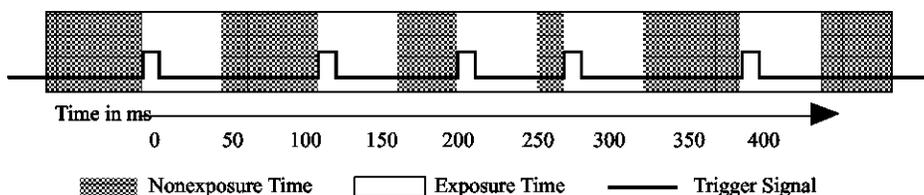
In `STROBED_MODE`, `pl_exp_start_seq` starts the camera. The camera enters clear mode while it waits for the first trigger signal to start the first exposure. As shown in the diagram above, each new exposure waits for an external trigger signal. Notice that the intervals between exposures can vary greatly, but the exposure times are constant.
