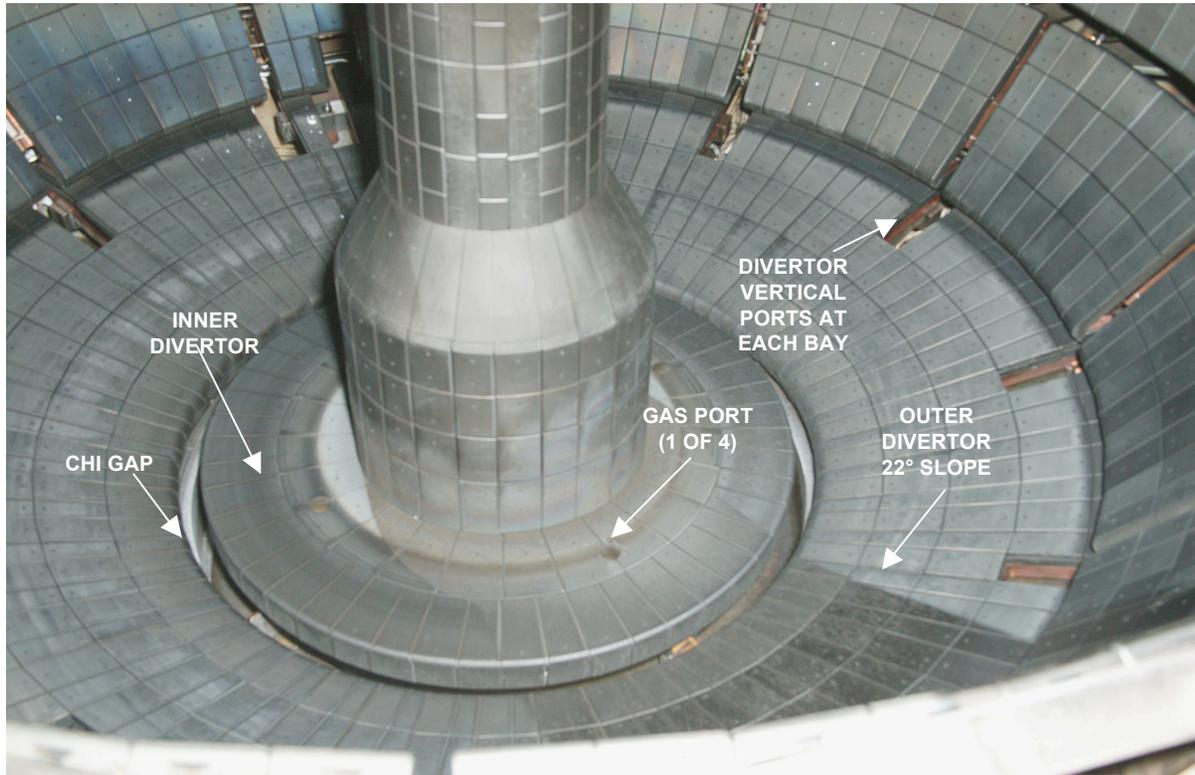
Photo of Lower Divertor after Lithium Evaporation
