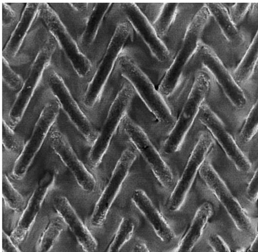
Fig. 1. Lithium-filled CPS surface view after one plasma pulse.
