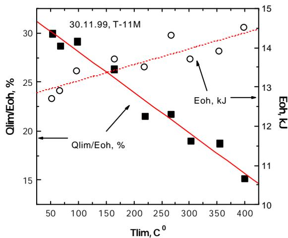
FIG. 2. Behaviour of relative energy incoming to limiter  $Q_{\text{lim}}/E_{\text{oh}}$  versus preheating temperature of limiter in ohmic mode.  $E_{\text{oh}}$  – total ohmic energy of discharge.
