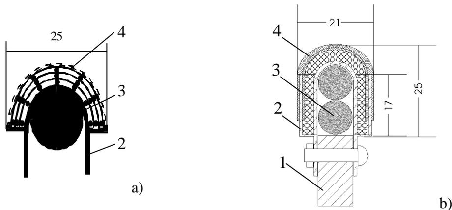
FIG. 1. Lithium limiter of T-11M tokamak:receiving element section of variant 1 (a) and variant 2 (b); 1-support, 2-case, 3-heater, 4- CPS.
