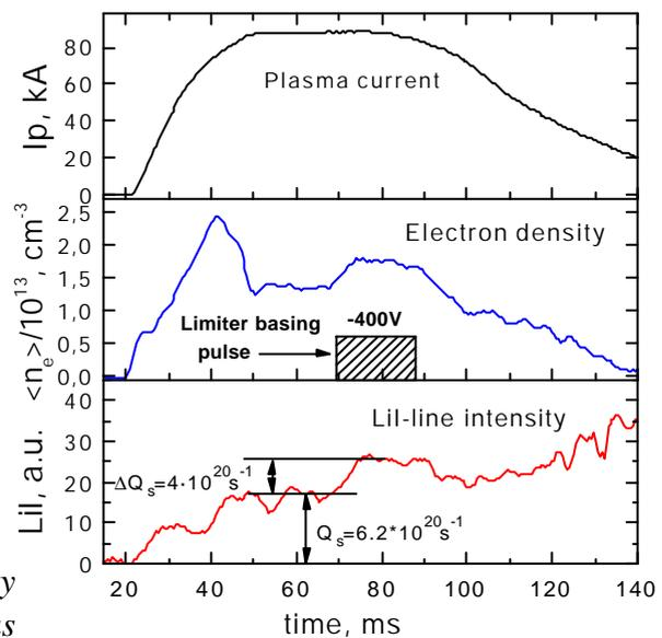
FIG. 3. Experimental evaluation of liquid Li sputtering yield by  $D^+$  ions from limiter.
